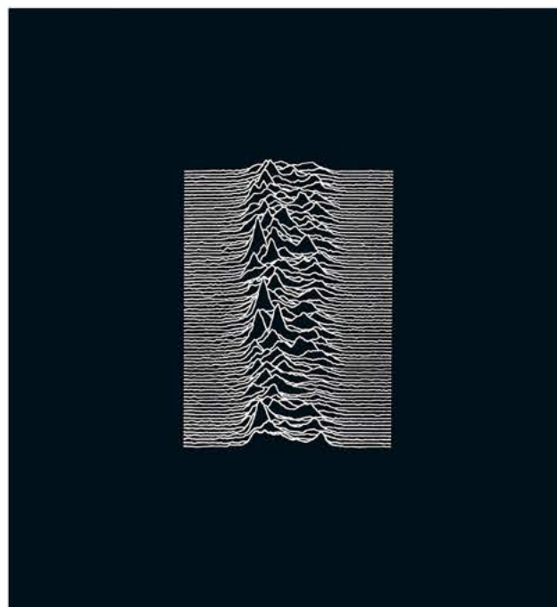
6.7: Successive pulses from the first pulsar discovered, CP 1919, are here superimposed vertically. The pulses occur every 1.337 seconds. They are caused by a rapidly-spinning neutron star.
